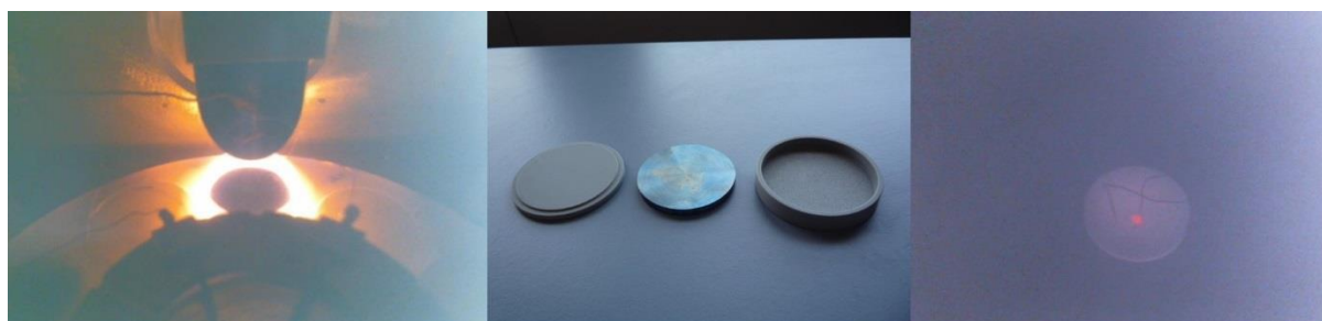
Figure 26 - Left: Webcam picture of steel disk glowing when heated above 700K. Centre: Steel disk and the ceramic enclosure used to mask its glowing in visible spectral range. Right: Webcam picture for the ceramic enclosure heated at 750K. The ceramic enclosure is slightly emitting in the visible spectral range, but much lower than the steel disk used previously.
