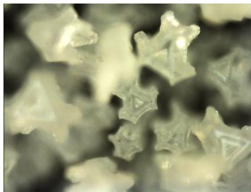
Figure 10- Microscope images.(left) CO 2 ice depositing as transparent slab ice and beginning to immerse sand under Martian conditions and (right) shows as yet un-researched crystal forms created at even lower temperatures and pressures
