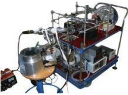
Serac cell and its thermodynamic system
