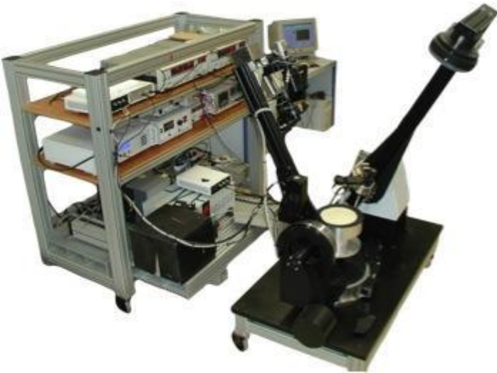
Spectro-Gonio Radiometer with its stabilized monochromatic source, the goniometer with illumination mirror, an open sample holder with sulfur powder and the detectors and the goniometer and detection electronics.
