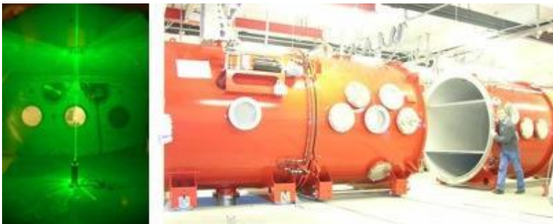
Green laser being used to monitor particle flow inside the chamber, b with Jon Merrison for scale
