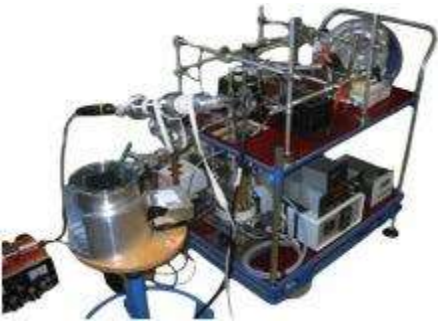
Serac cell and its thermodynamic system
